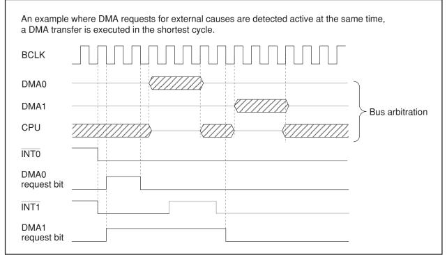
Figure 11.6 DMA Transfer by External Factors
